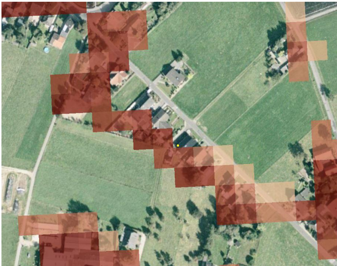
Figure 15: Different scale and geometric resolutions lead to a potential mismatch of LUCAS sample point (yellow, LC=Axx) and IMD product (red pixels indicating %imperviousness)
