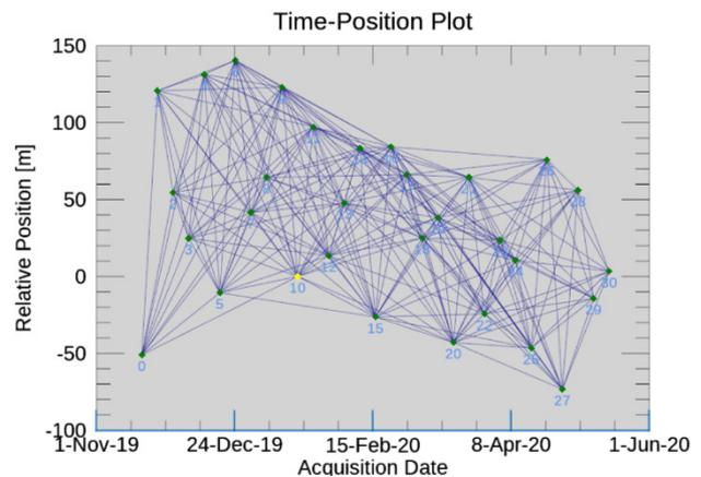
Figure 5. Normal and temporal baselines of connected image pairs in SBAS processing.
