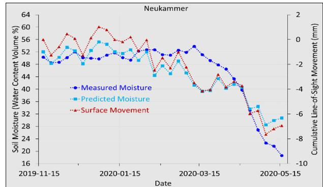
Figure 9. Comparison of soil moisture and SBAS-derived movement at Neukammer (Figure 3).
