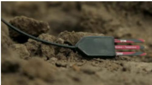
Figure 2. Decagon 5TM to measure underground soil moisture (<https://www.ictinternational.com/products/5tm/decagon-5tm-vwc-temp/>)
