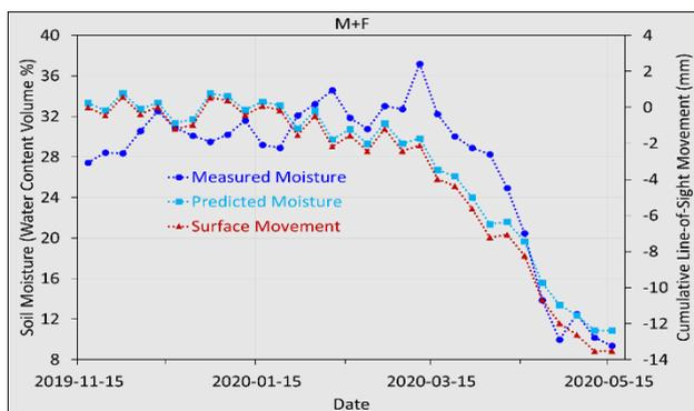
Figure 8. Comparison of soil moisture and SBAS-derived movement at M+F (Figure 3).
