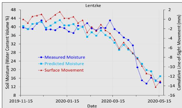
Figure 7. Comparison of soil moisture and SBAS-derived movement at Lentzke (Figure 3). Movement: negative and positive, away and towards Sentinel-1 antenna. Sample dates correspond to Sentinel-1 acquisitions.
